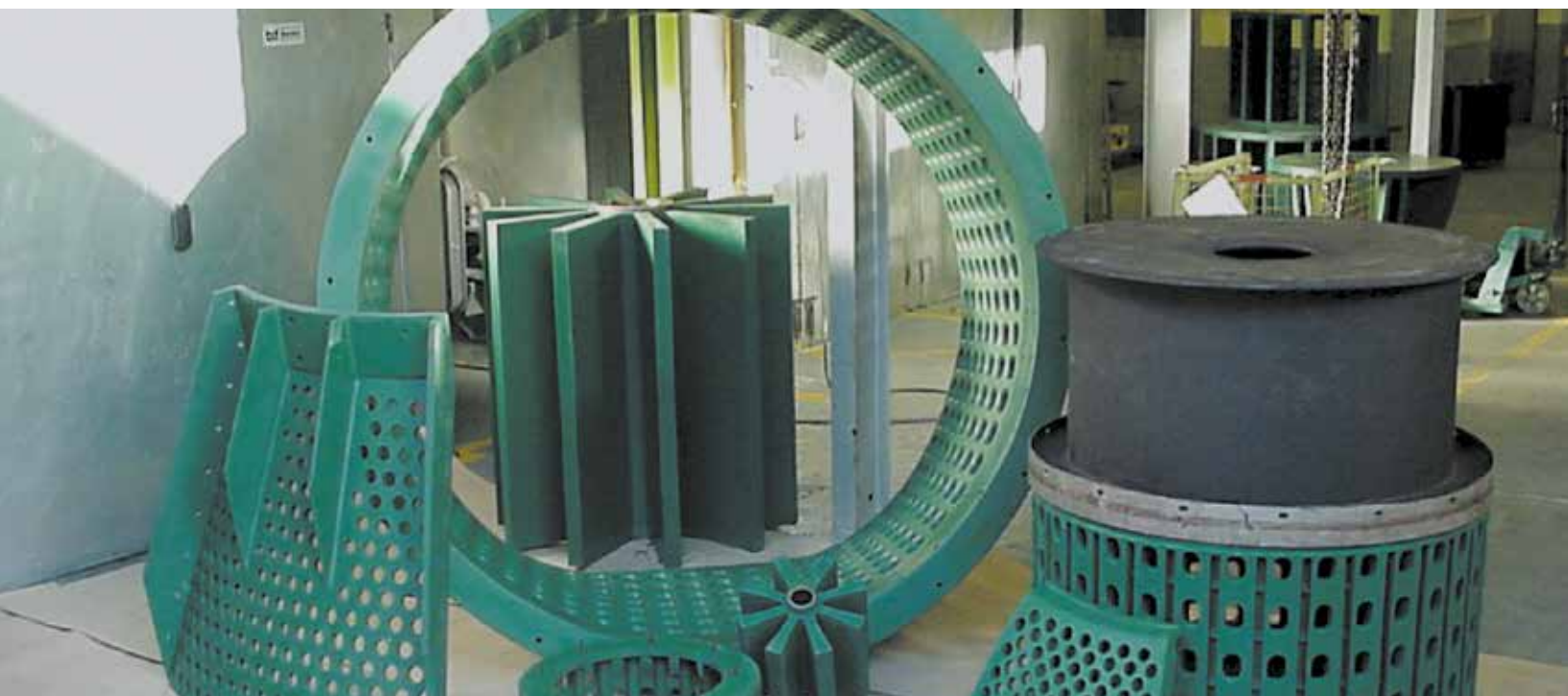
Rotors, Dispersers, Hoods and Standpipes
